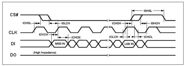
Figure 31. Input Timing
