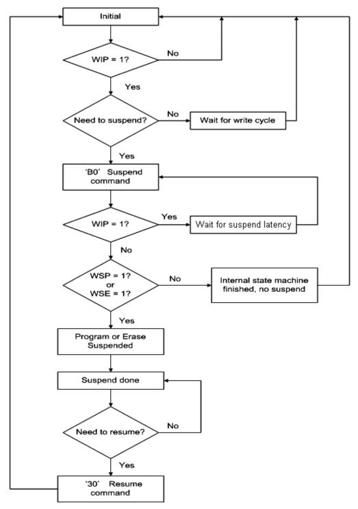
Figure 27.2. Write Suspend/Resume Flow
