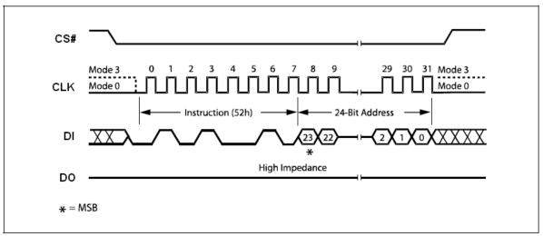
Figure 29. 32KB Half Block Erase Instruction Sequence Diagram
