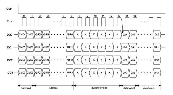
Figure 16.1 Fast Read Instruction Sequence in QPI Mode
