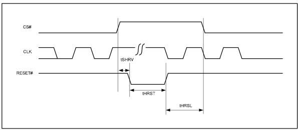
Figure 33. Reset Timing
