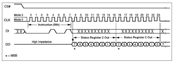
Figure 12. Read Status Register 2 Instruction Sequence Diagram
