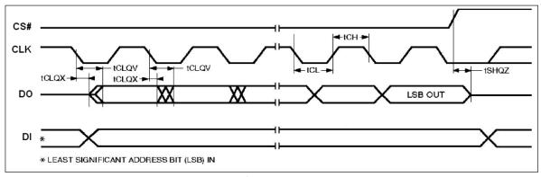
Figure 30. Serial Output Timing
