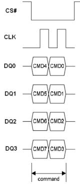
Figure 27.1. Write Suspend/Resume Instruction Sequence in QPI Mode
