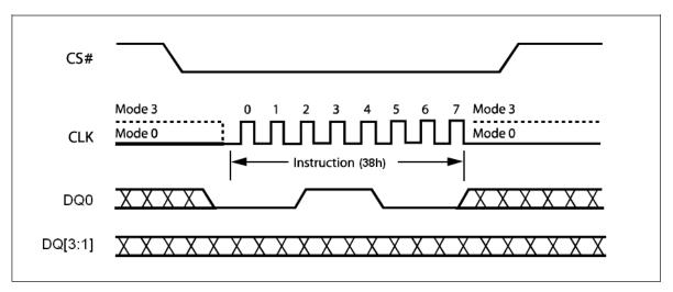
Figure 7. Enable Quad Peripheral Interface mode Sequence Diagram
