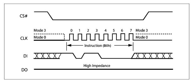
Figure 25. Write Suspend Instruction Sequence Diagram
