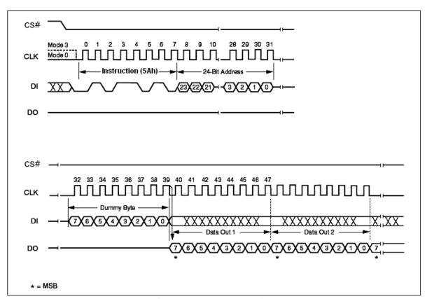
Figure 38. Read SFDP Mode Instruction Sequence Diagram
