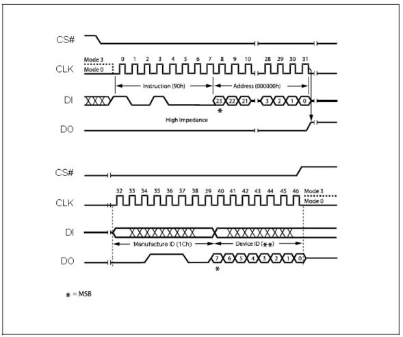
Figure 35. Read Manufacturer / Device ID Diagram
