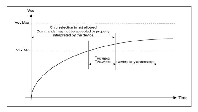
Figure 28. Power-up Timing
