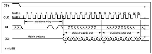
Figure 11. Read Status Register Instruction Sequence Diagram
