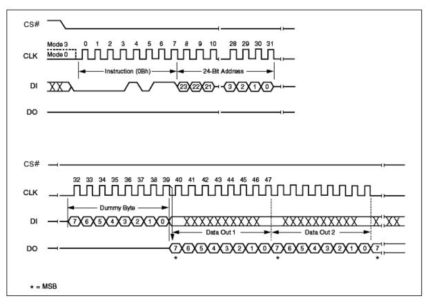
Figure 16. Fast Read Instruction Sequence Diagram
