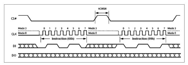
Figure 6. Reset-Enable and Reset Sequence Diagram
