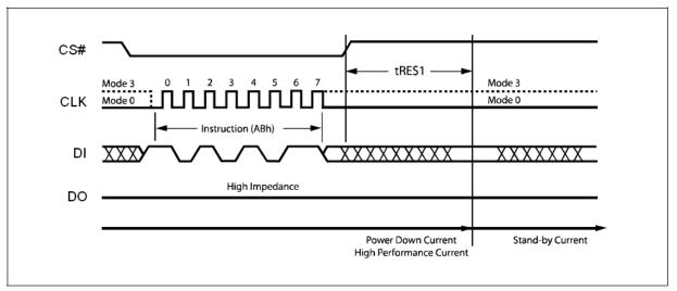
Figure 33. Release Power-down Instruction Sequence Diagram
