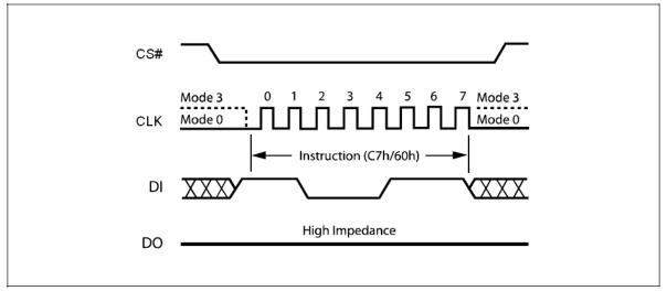
Figure 31. Chip Erase Instruction Sequence Diagram
