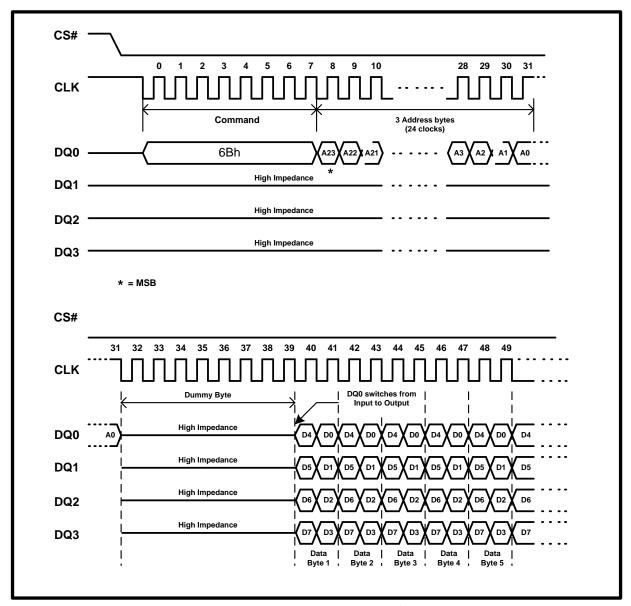
Figure 19. Quad Output Fast Read Instruction Sequence Diagram
