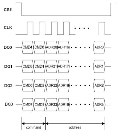
Figure 30.1 Block/Sector Erase Instruction Sequence in QPI Mode
