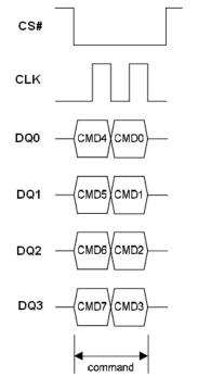
Figure 37.1 Enter OTP Mode Sequence in QPI Mode
