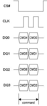
Figure 31.1 Chip Erase Sequence in QPI Mode
