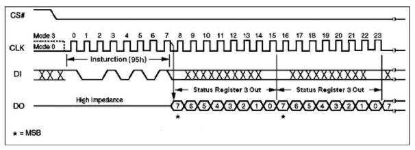
Figure 13. Read Status Register 3 Instruction Sequence Diagram
