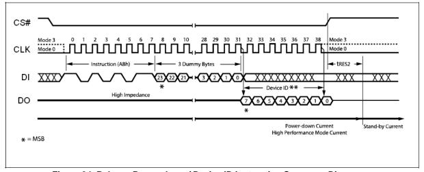
Figure 34. Release Power-down / Device ID Instruction Sequence Diagram
