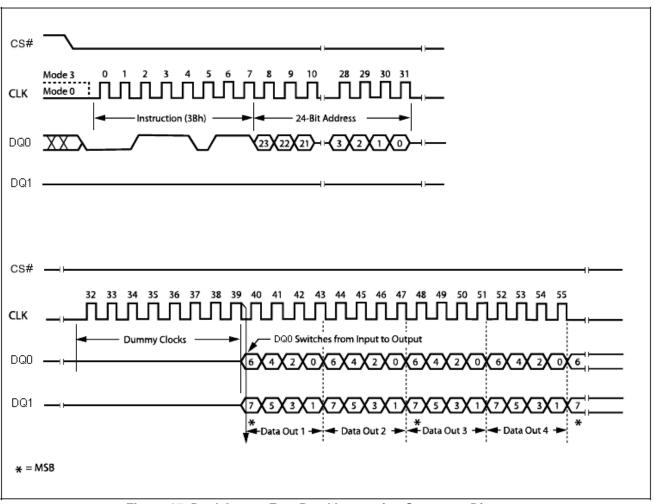
Figure 17. Dual Output Fast Read Instruction Sequence Diagram
