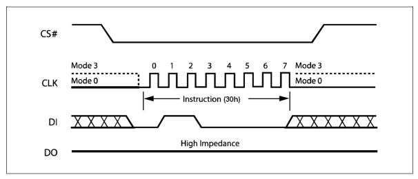
Figure 27. Write Resume Instruction Sequence Diagram
