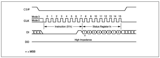
Figure 14. Write Status Register Instruction Sequence Diagram
