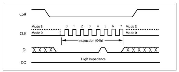
Figure 10. Write Disable Instruction Sequence Diagram
