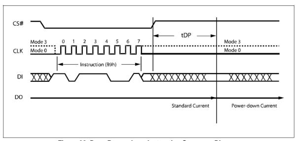
Figure 32. Deep Power-down Instruction Sequence Diagram
