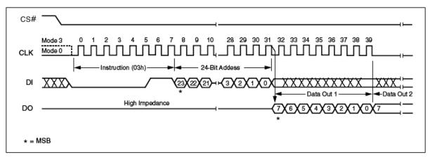
Figure 15. Read Data Instruction Sequence Diagram
