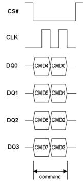
Figure 10.1 Write Enable/Disable Instruction Sequence in QPI Mode
