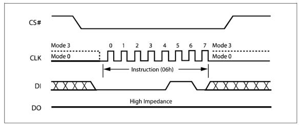
Figure 8. Write Enable Instruction Sequence Diagram
