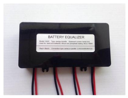
HA02 battery equalizer is energy transfer type equalizer, it can compensate for batteries with two sides. The equalizer starts to work when there are 10mV between two batteries. The current will flow from a higher voltage to low voltage, eventually reach equilibrium. It can connect with battery system with 24 hours, to keep the system energy balance automatically, no need manual maintenance.
