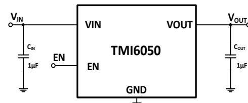
Figure 2. TMI6050 fixed output Circuit
