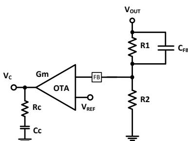
Figure 5. Application Circuits of Feedforward Capacitor  $C_{FB}$
