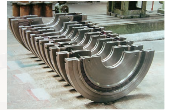
steam turbine bulkhead
