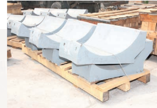
grinding track segments
