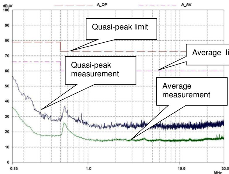
**Figure 3 Conducted Emission 200 V, 0.75 kW model, 3 kHz switching frequency, 50 m cable, filter part No. 4200-1000**
