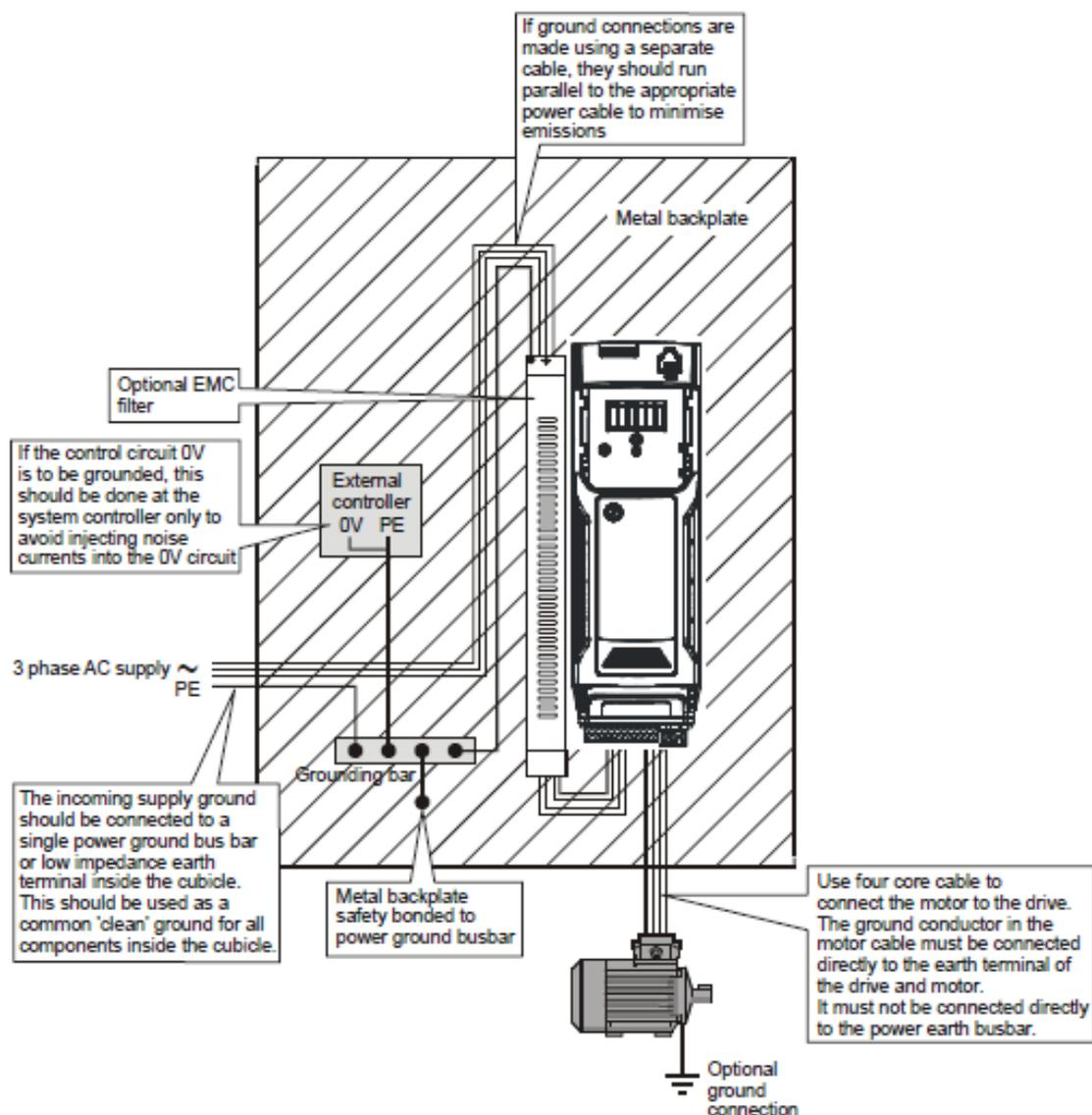
Figure 4 Wiring guidelines
