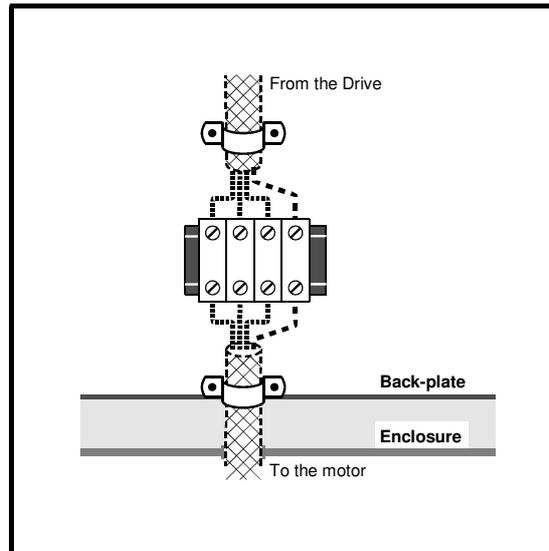
Figure 5 Arrangement for terminal block in motor cable
