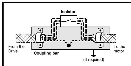
Figure 6 Arrangement for isolator switch in motor cable
