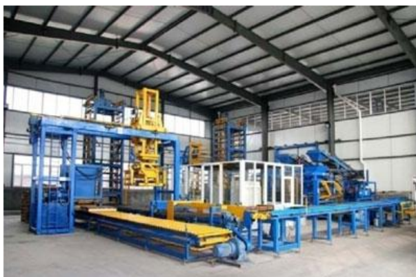
Pictured –Fully Automatic Block Production Line
