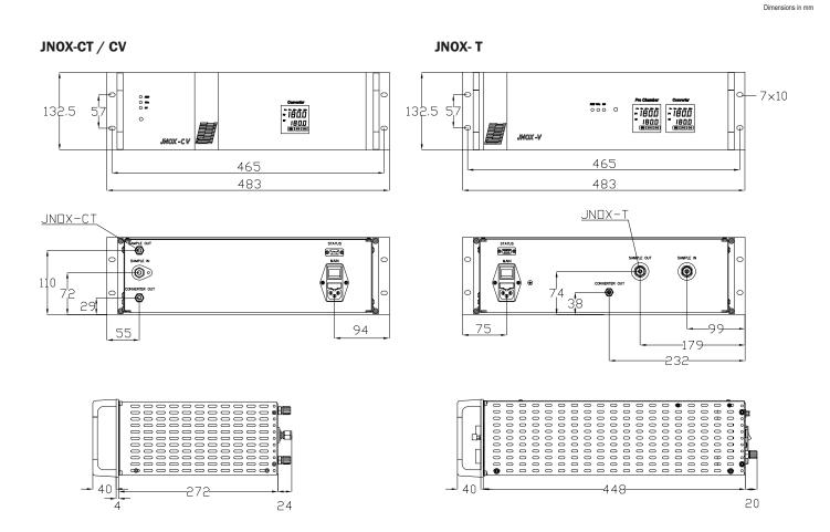
JNOX-CTW / CVW / TW / CTP / CVP / TP in portable (P) or wall mounting housing (W)
