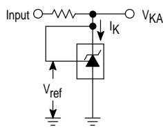
**Figure 2. Test Circuit for  $V_{KA} > V_{\text{ref}}$**
