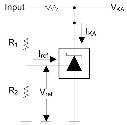
Test Circuit for  $V_{\text{KA}} = V_{\text{ref}}(1 + R_1/R_2) + R_1 \cdot I_{\text{ref}}$
