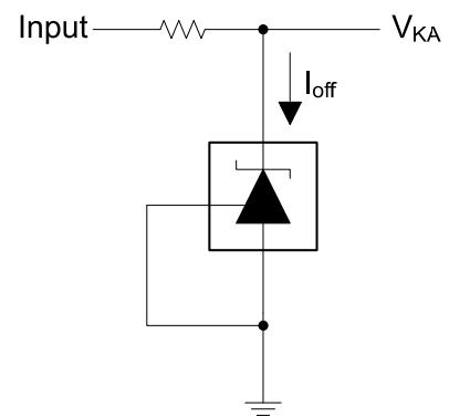
Test Circuit for  $I_{\text{off}}$
