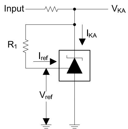
Test Circuit for  $I_{\text{ref}}$
