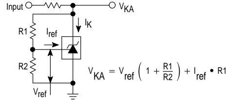
**Figure 3. Test Circuit for  $I_{\text{off}}$**
