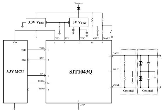
Fig 13 Typical application with 3.3V MCU
