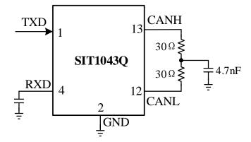
Fig 11 Transceiver bus symmetry test circuit
