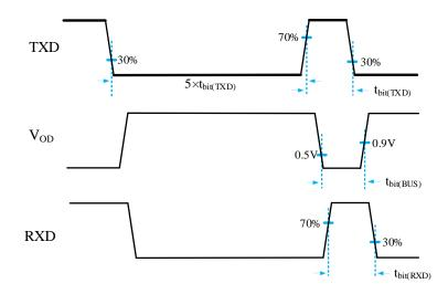
Fig 8 tbit timing diagram
