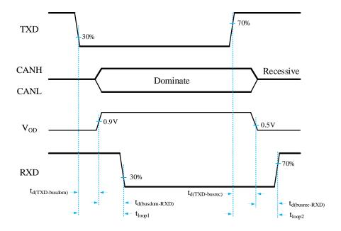
Fig 7 CAN transceiver timing diagram
