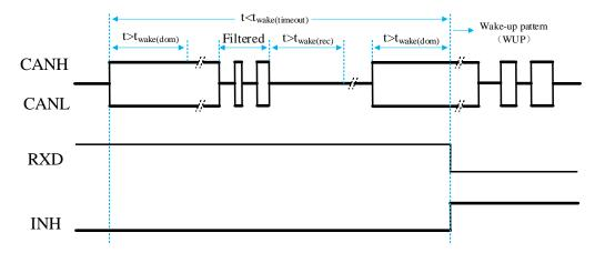
Fig 5 Remote wake-up diagram
