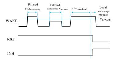
Fig 3 Local wake-up for WAKE rising edge
