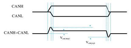
Fig 9 CAN bus common-mode voltage (according to SAE 1939-14)
