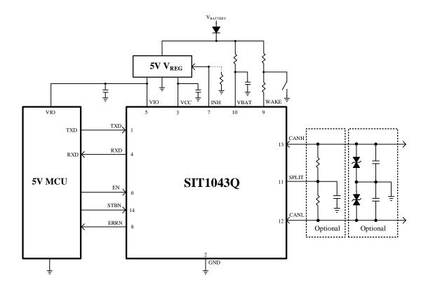
Fig 12 Typical application with 5V MCU
