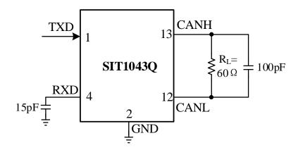
Fig 10 Transceiver timing sequence test circuit
