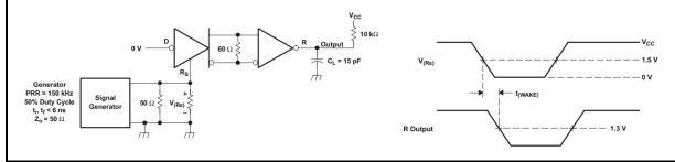
Fig 7 t<sub>(WAKE)</sub> test circuit and waveform
