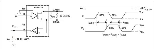
The input pulse is supplied by a generator having the following characteristics: PRR≤125kHz, 50% duty cycle, tr<6ns, tr<6ns.
