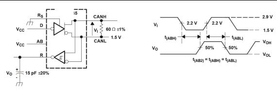
The input pulse is supplied by a generator having the following characteristics: PRR≤125kHz, 50% duty cycle, t<sub>r</sub><6ns, t<sub>f</sub><6ns.
