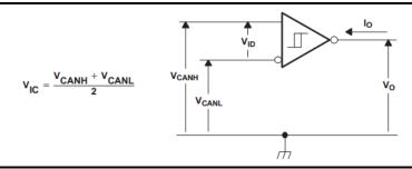
Fig 5 Receiver voltage and current definitions
