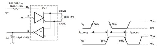
The input pulse is supplied by a generator having the following characteristics:  $PRR \leq 125 kHz, 50\% \ duty \ cycle, \ t_{i} \leq 6ns, \ t_{i} \leq 6ns, \ Zo = 50\Omega.$
