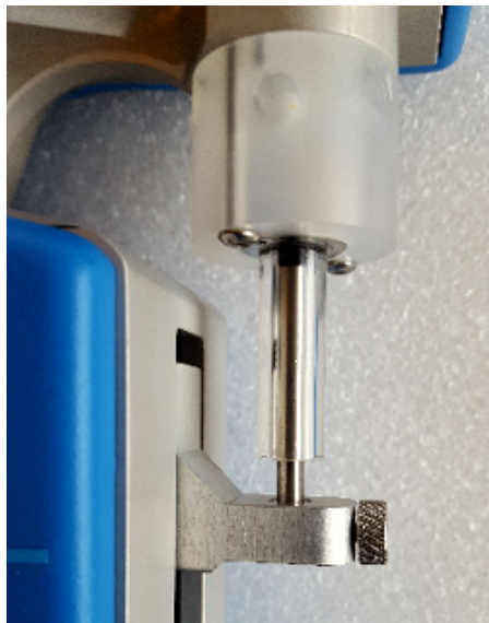
FIGURE 4.5 – Correct plunger lock screw fixation
