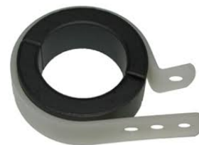
FIGURE 2.2 – Ferrite 600 04 27 from Sibalco to be added with 4 loops around the power cable
