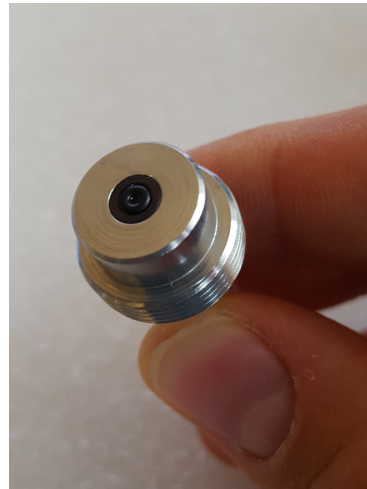
FIGURE 4.3 – Syringe seal to be handled with care. Before screwing the syringe, ensure that the black O-ring is correctly inserted in the groove as shown here
