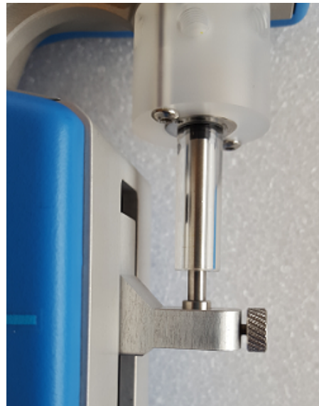
FIGURE 4.6 – Incorrect plunger lock screw fixation
