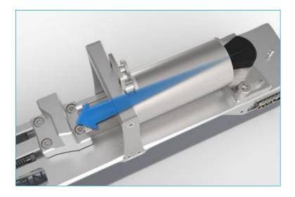
Lock the syringe piston with the knurled screw. To avoid bending the syringe in case of high pressure, lower the blank holder onto the syringe and fasten the two knurled screws.
