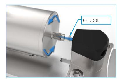
In order to make use of the entire syringe volume, move the piston holder to the front position through the software. Push back the syringe holder until the piston touches the piston holder. Retighten the fastening screws of the syringe holder.
