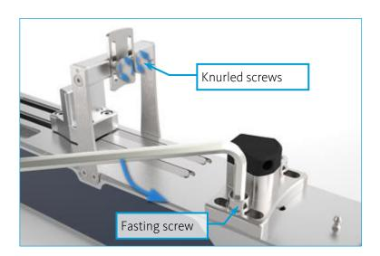
Screw the syringe into the syringe holder. Use one of the supplied PTFE disks to achieve a sealed connection.
