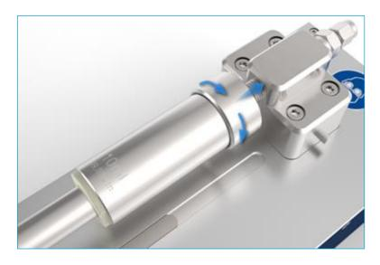
Put the safety hood back on the device and advance the piston holder until it touches the piston. Take off the safety hood and attach the piston to the piston holder using the knurled screw.
