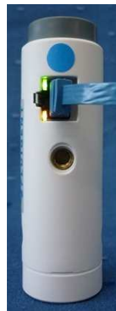
Orange indicator + green indicator (Power OK + Check connection)
