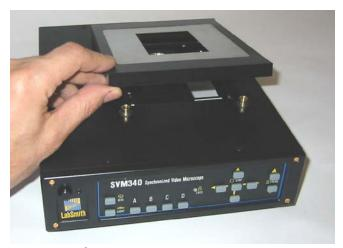
Removing the microscope stage
