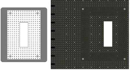
Integrating Delrin stage shown assembled with LS600-CH (left) and iBB (right) breadboards
