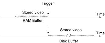
Pre-trigger (top) and post-trigger (bottom) recording
