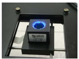
Illumination module installed in SVM340
