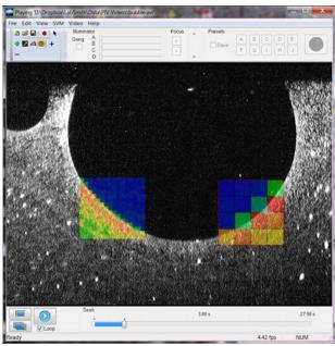
Example of macropixel probes. Probe on left had array of 8 x 8 pixel size; probe on right has 32 x 32 pixel size.
