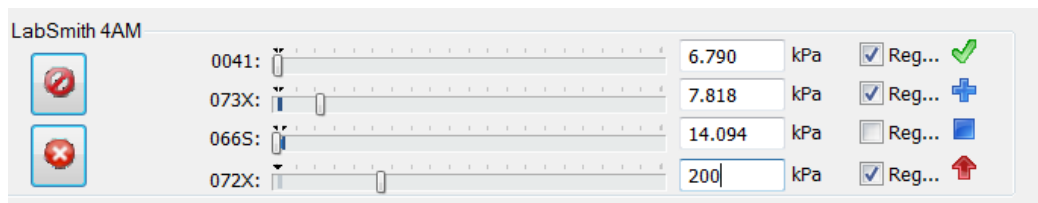
Figure 13 Typical Control Overview Window view of analog manifold controls.
