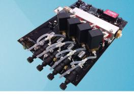
The multi-channel design is highly compact, ranging from 1 to 4 channels for the P-OEM series and from 5 to 8 channels for the PL-OEM series. Since fluids are not in contact with the instrument, there is no routine cleaning and contamination is drastically reduced.
