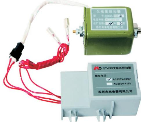
In the electrified wire netting where thunder and rain often happens or whose power supply is not stable, undervoltage release with time delay is recommended to protect circuit breaker from releasing by transient voltage-lowering. Delay time is 1s, 2s, 3s, 5s. It is selective by customers.
