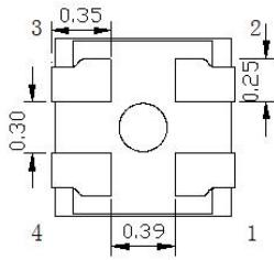
For reflow soldering
