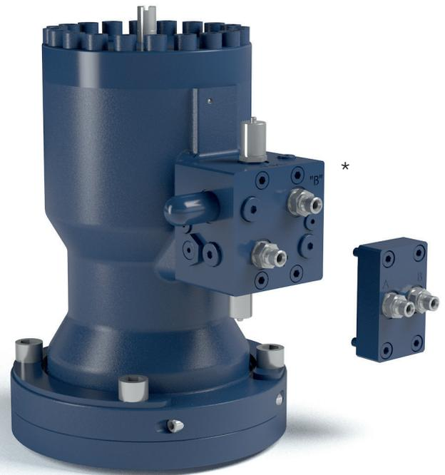
\*Hydraulic control block ensures containment of hydraulic pressure inside the actuator in case of damage to hydraulic lines and can be used to adjust hydraulic pressure input of individual actuators.
