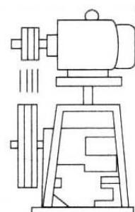
G with flexible coupling and geared motor
