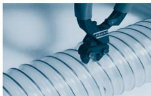
Step 2: Snip the supporting spiral with wire pliers.
