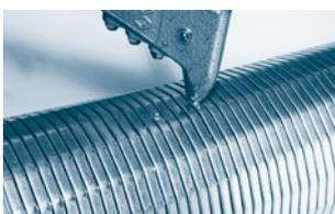
Step 1: Fix the ends with rivets or by soldering.
