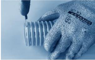
Step 3: Cut round ¼ of the hose wall next to the wire, leaving the wire in the detached part of the hose wall.
