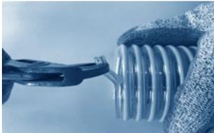
Step 4: Grip the detached strip of hose wall and pull until the grounding wire is exposed.
