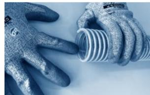
For grounding, bend the grounding wire into the hose and insert the conductive hose fitting to be earthed.
