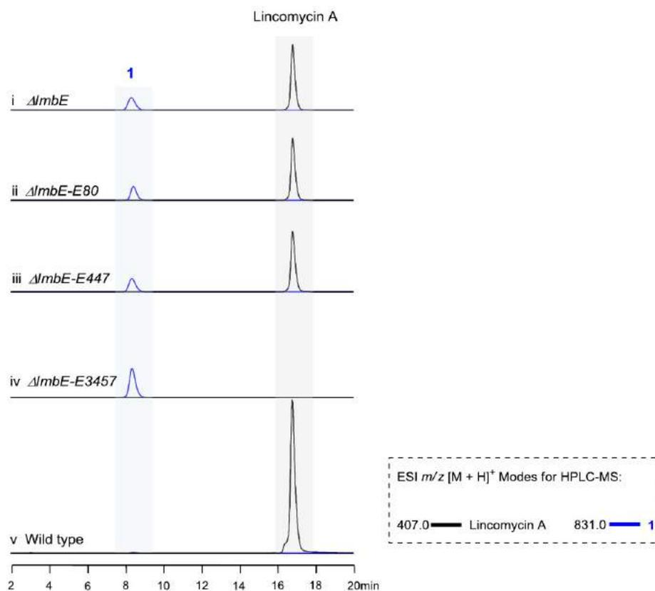
**Extended Data Figure 3 | The production of MSH S-conjugate 1 and lincomycin A in various *S. lincolnensis* strains.** The strains include the mutants (i, for  $\Delta lmbE$ ; ii, for  $\Delta lmbE-E80$ ; iii, for  $\Delta lmbE-E447$ ; and iv, for
